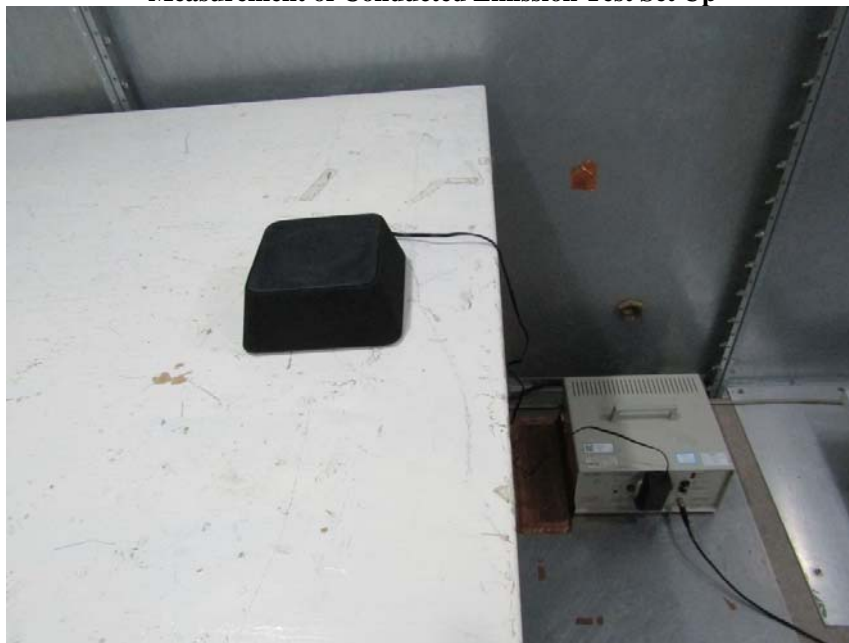
Measurement of Conducted Emission Test Set Up
