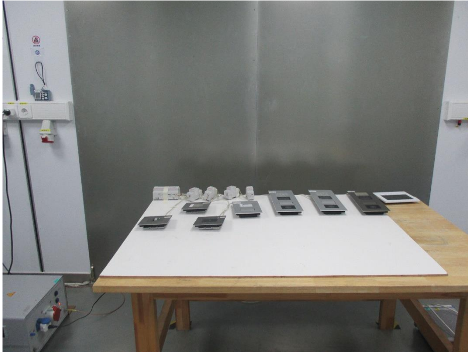
Setup photo of conducted emission (150KHz-30MHz)
