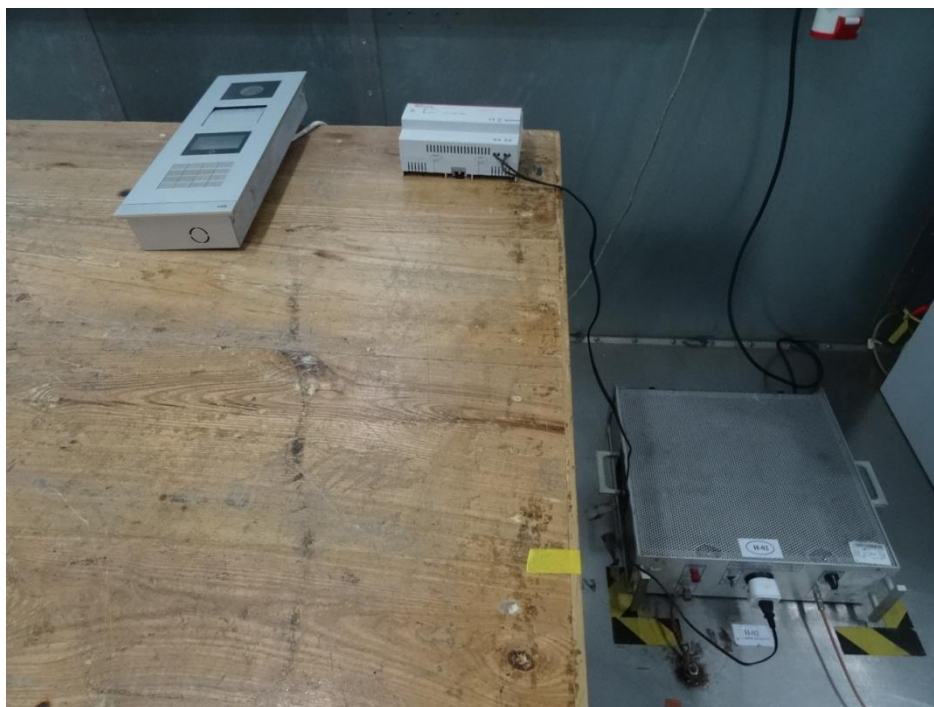
Setup photo of conducted emission (150KHz-30MHz)
