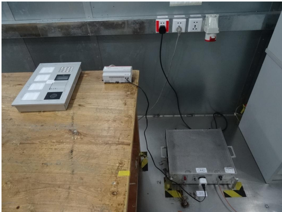
Setup photo of conducted emission (150KHz-30MHz)
