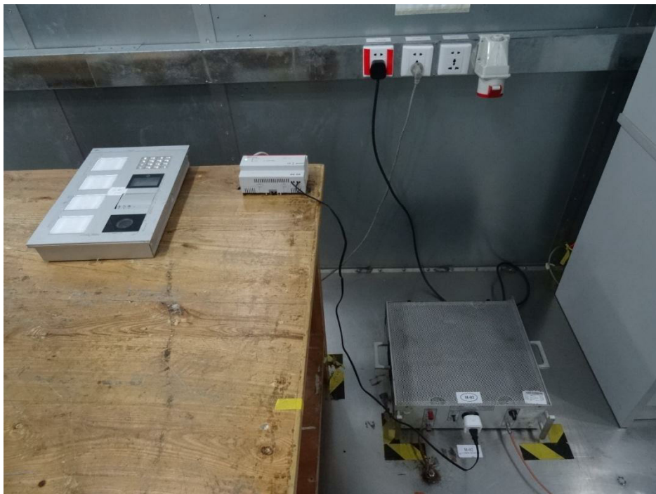
Setup photo of conducted emission (150KHz-30MHz)
