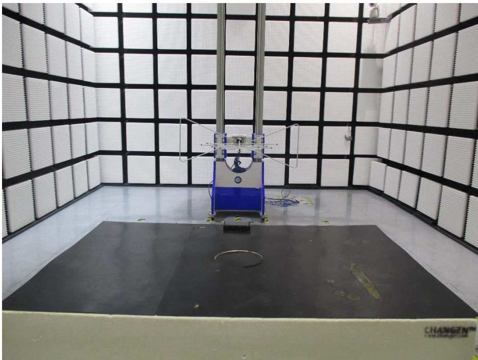
Setup photo of radiated emission (30MHz-1GHz)
