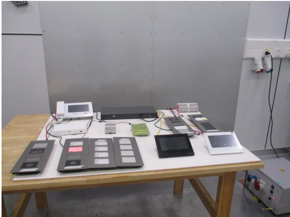
Setup photo of conducted emission (150KHz-30MHz)
