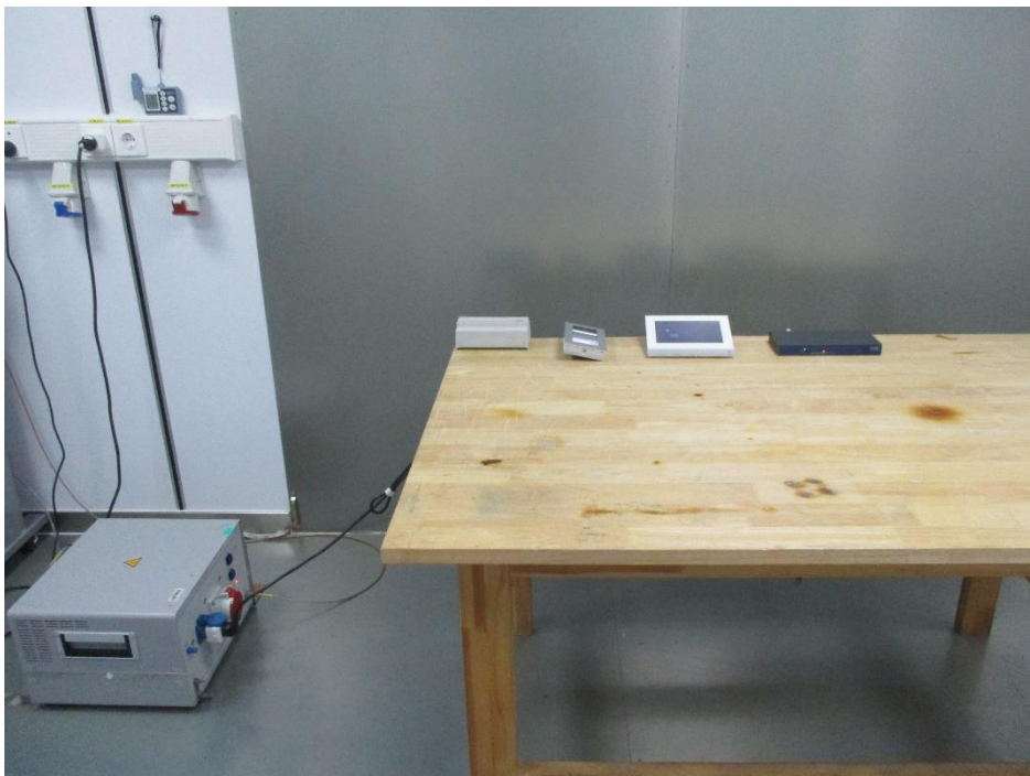
Setup photo of conducted emission (150KHz-30MHz)
