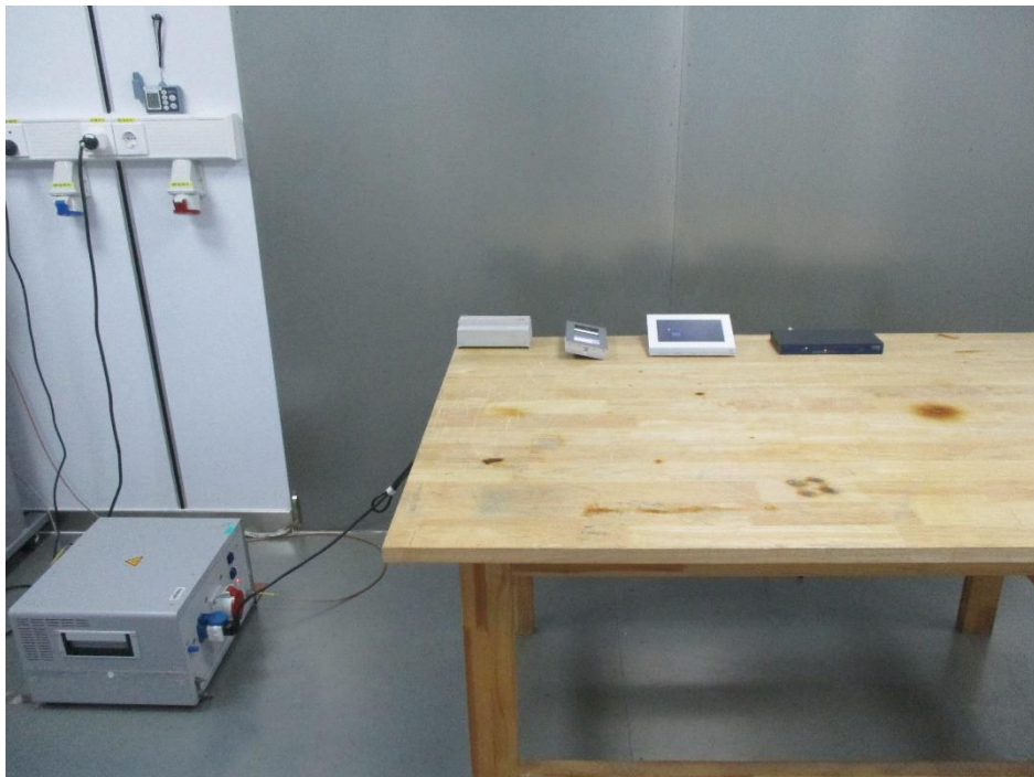
Setup photo of conducted emission (150KHz-30MHz)
