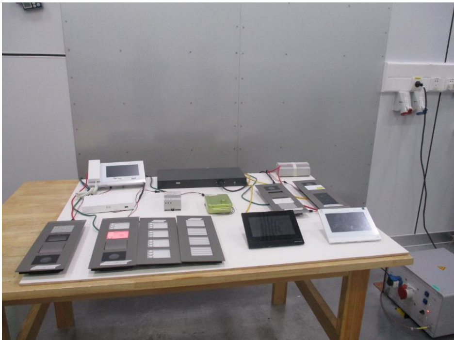
Setup photo of conducted emission (150KHz-30MHz)
