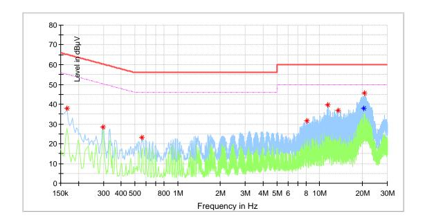
No significant emission was detected within 10 dB to limit
