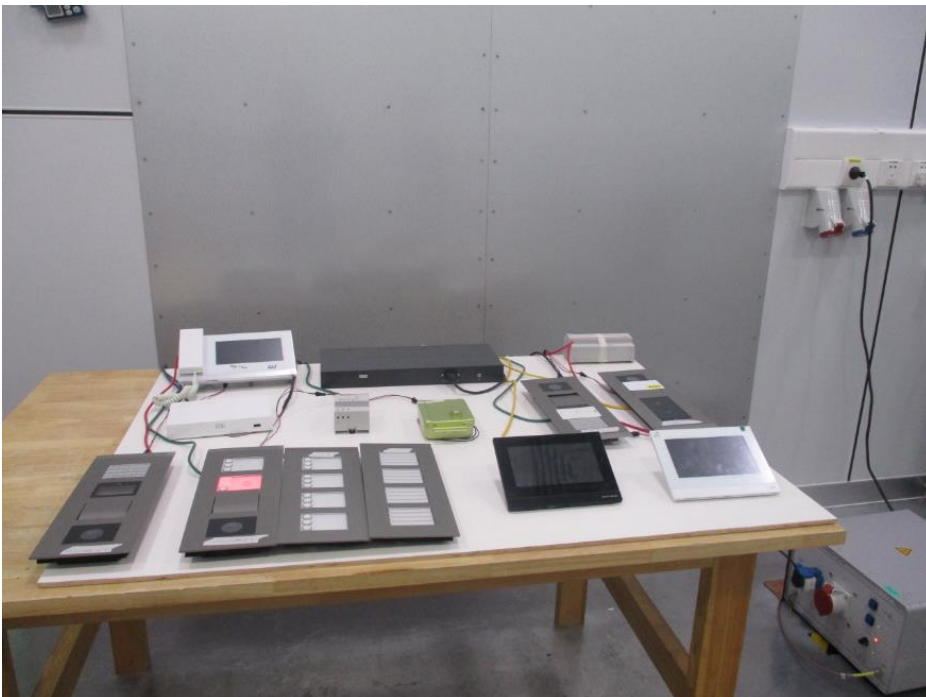
Setup photo of conducted emission (150KHz-30MHz)
