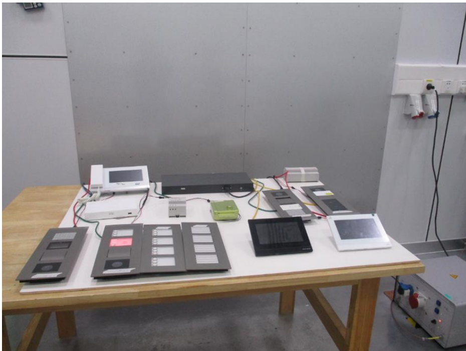
Setup photo of conducted emission (150KHz-30MHz)
