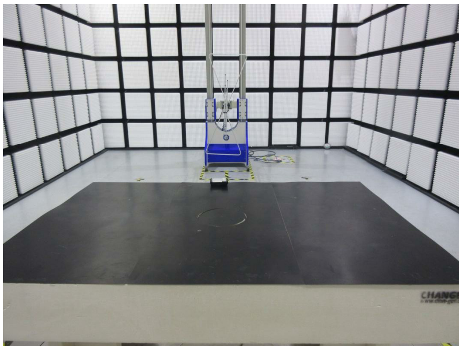
Setup photo of radiated emission (30MHz-1GHz)
