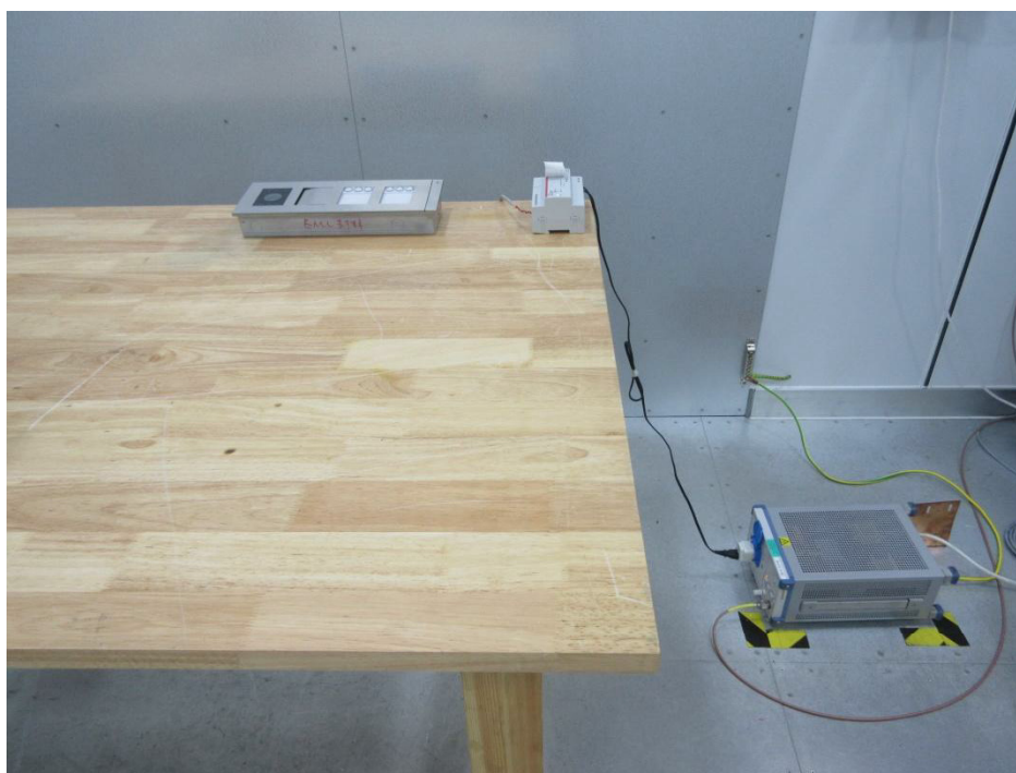
Setup photo of conducted emission (150KHz-30MHz)
