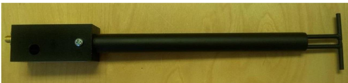
Figure 1 – MVG COMOSAR Validation Dipole
