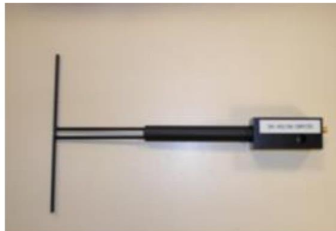
Figure 1 – Satimo COMOSAR Validation Dipole
