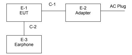
Radiated Spurious Emission Test
