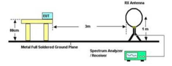
(B) Radiated Emission Test-Up Frequency 30MHz~1GHz
