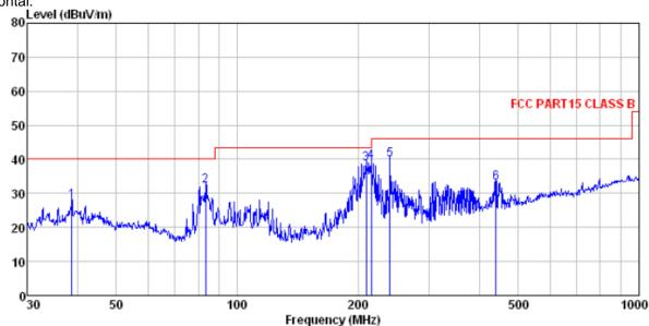
Site : 3m chamber Condition : FCC PART15 CLASS B 3m VULB9163-2013M HORIZONTAL ReadAntenna Cable Preamp Limit Loss Factor Level Line Limit Remark Freq Level Factor dBu∀ dB/m ₫B dB dBuV/m dBuV/m MHz 38.752 43.78 15.25 0.65 32.06 27.62 40.00 -12.38 QP 51.00 11.87 1.06 2 83.522 31.75 32.18 40.00 -7.82 QP 209.313 215.268 1.89 3 12.87 38.60 43.50 -4.90 QP 55.98 32.14 4 43.50 -4.36 QP 46.00 -6.22 QP 56.33 55.78 13.03 39.14 1.93 32.15 5 239.987 14.09 2.07 32.16 39.78
