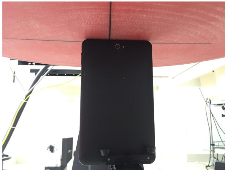
Test Position 4 - Body-worn, the top side of the EUT towards ground (The distance was 0mm)
