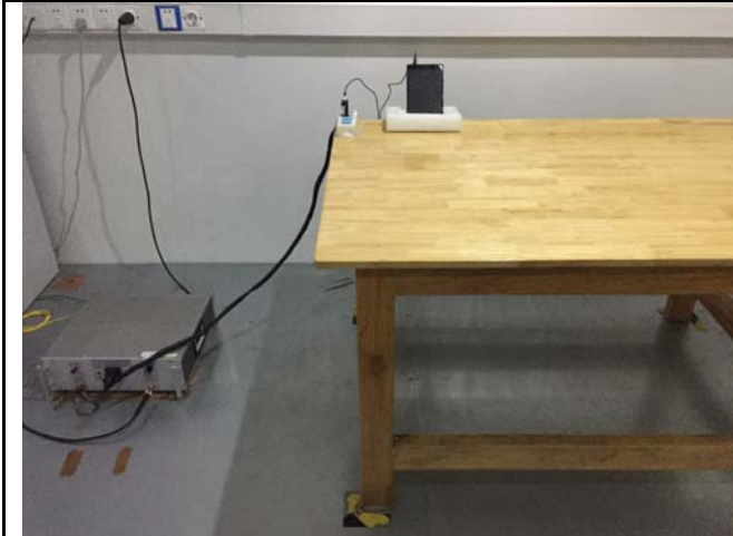
Conducted Emissions Test Setup Front View
