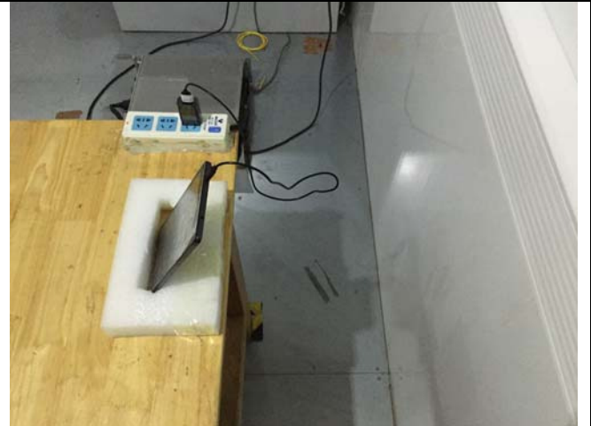
Conducted Emissions Test Setup Side View
