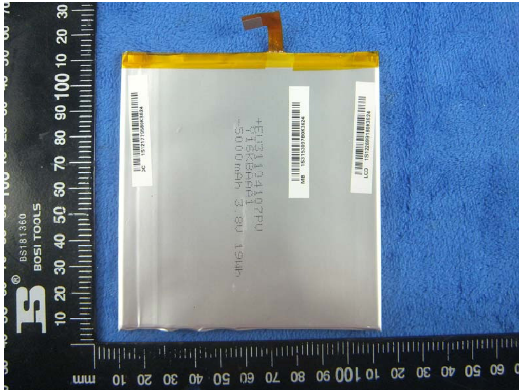
Battery - Front View
