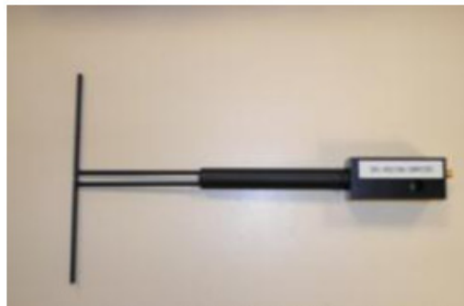
Figure 1 – Satimo COMOSAR Validation Dipole
