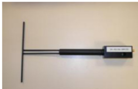
Figure 1 – Satimo COMOSAR Validation Dipole
