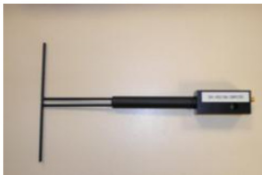
Figure 1 – Satimo COMOSAR Validation Dipole
