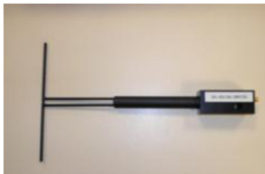
Figure 1 – Satimo COMOSAR Validation Dipole
