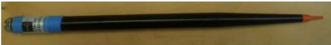
Figure 1 – MVG COMOSAR Dosimetric E field Dipole
