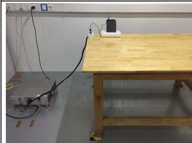
Conducted Emissions Test Setup – Front View ( MP4 mode )
