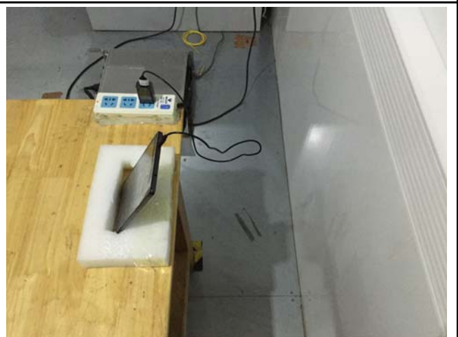
Conducted Emissions Test Setup – Side View ( MP4 mode )
