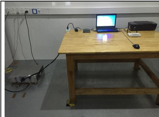
Conducted Emissions Test Setup – Front View ( USB mode )
