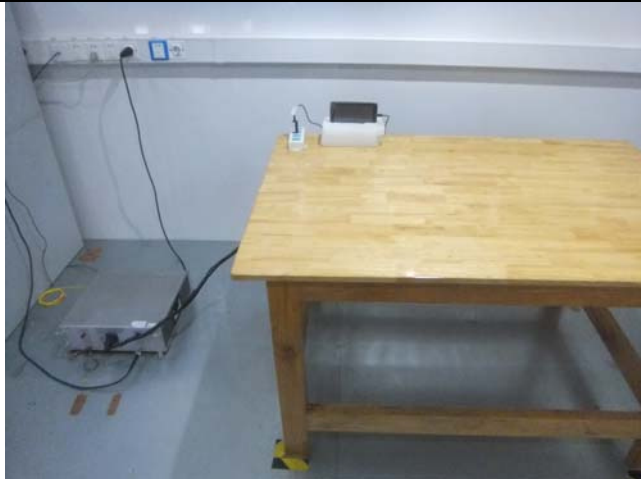
Conducted Emissions Test Setup Front View
