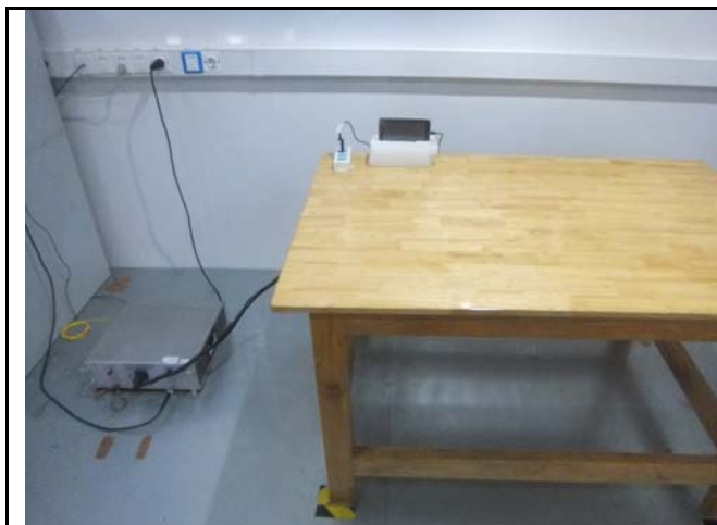
Conducted Emissions Test Setup Front View
