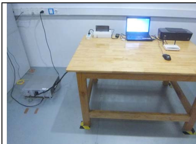
Conducted Emissions Test Setup – Front View
