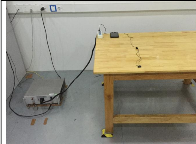
Conducted Emissions Test Setup – Front View
