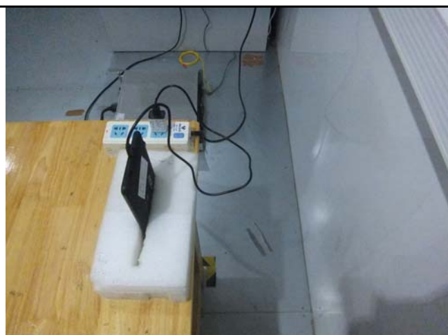
Conducted Emissions Test Setup Side View
