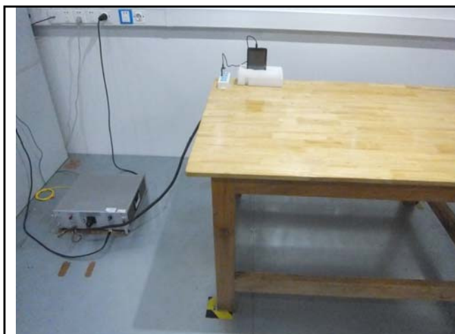
Conducted Emissions Test Setup Front View
