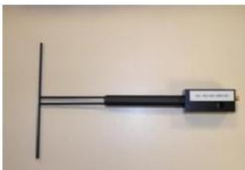
Figure 1 – Satimo COMOSAR Validation Dipole
