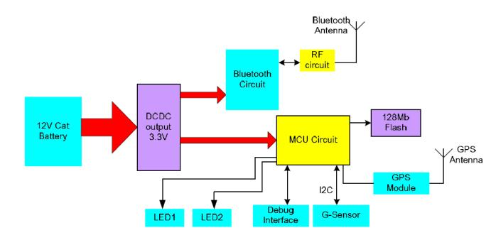
This product will be designed based on the STM32 Baseband chipset, which includes GPS functionality, Bluetooth LE, G-sensor. This baseband external connect a 128Mb serial flash.
