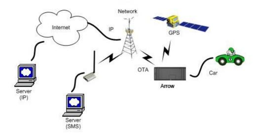
This product will be designed based on the MDM9207-1 baseband chipset, which includes LTE Cat.1, and GPS functionality. The device will use one multi-band antenna and one dedicated GPS antenna.
