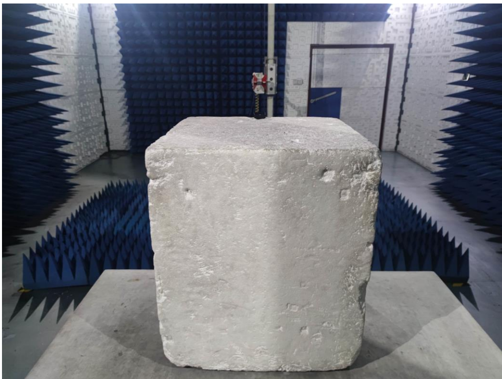
RADIATED EMISSION TEST SETUP ABOVE 1GHz
