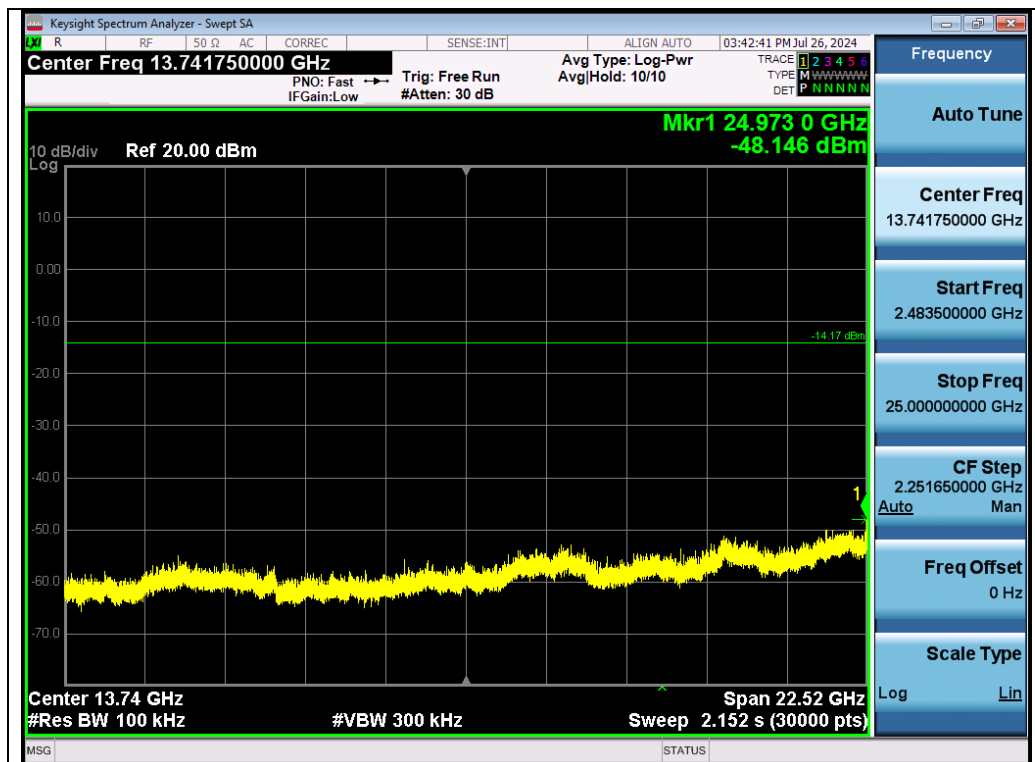
Test_Graph_LE1M_ANT1_2402_1Mbps_Higher Band Emissions
