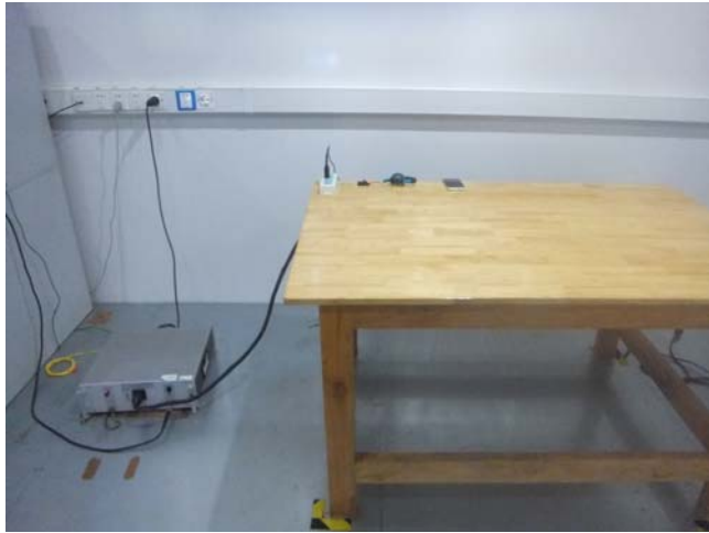
Conducted Emissions Test Setup – Front View
