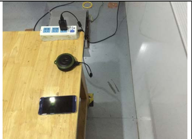
Conducted Emissions Test Setup Side View
