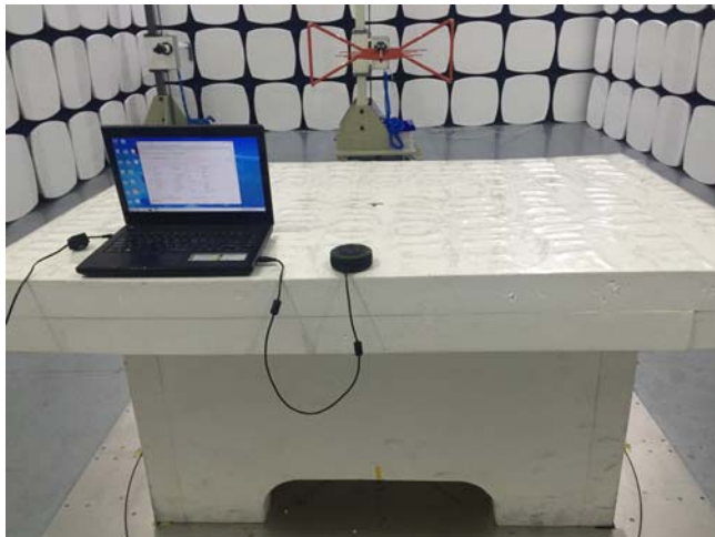
Conducted Emissions Test Setup Front View
