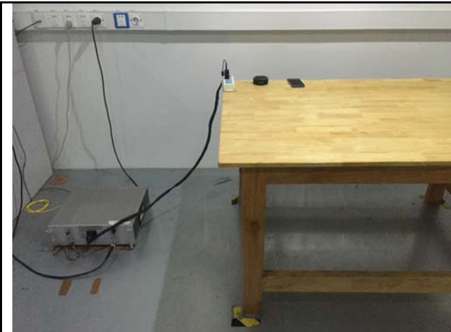
Conducted Emissions Test Setup Front View
