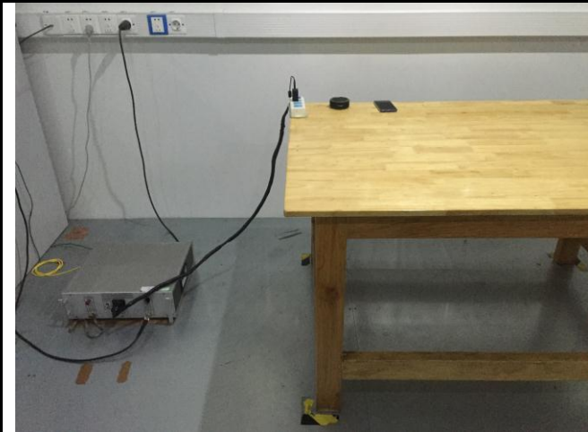
Conducted Emissions Test Setup Front View
