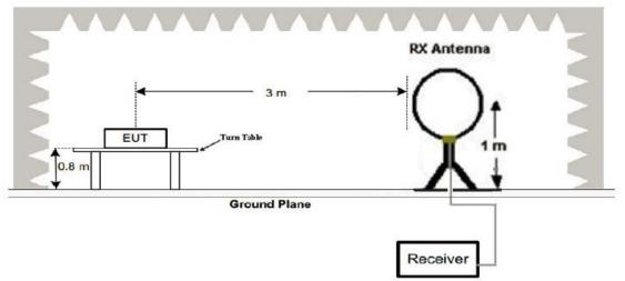
(2) Radiated Emission Test-Up Frequency 30MHz~1GHz
