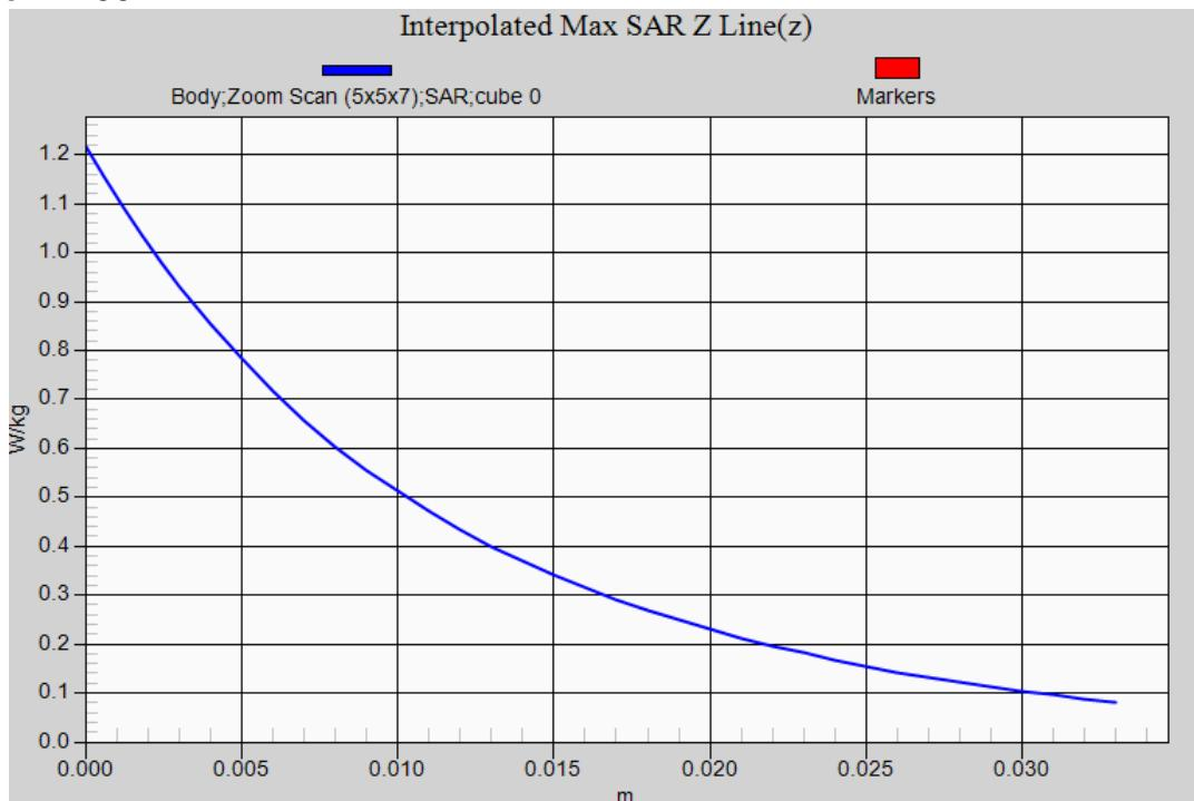
**WCDMA RMC Band 5 (Limbs SAR) EUT Right-side (0mm (Pwr OFF)) Z-Axis plot**
