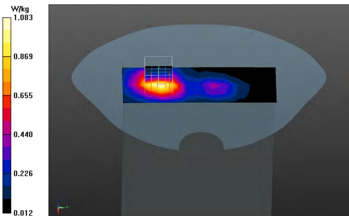
**1xEVDO BC1 (Body SAR) EUT Back (6mm (Pwr OFF)) Z-Axis plot
