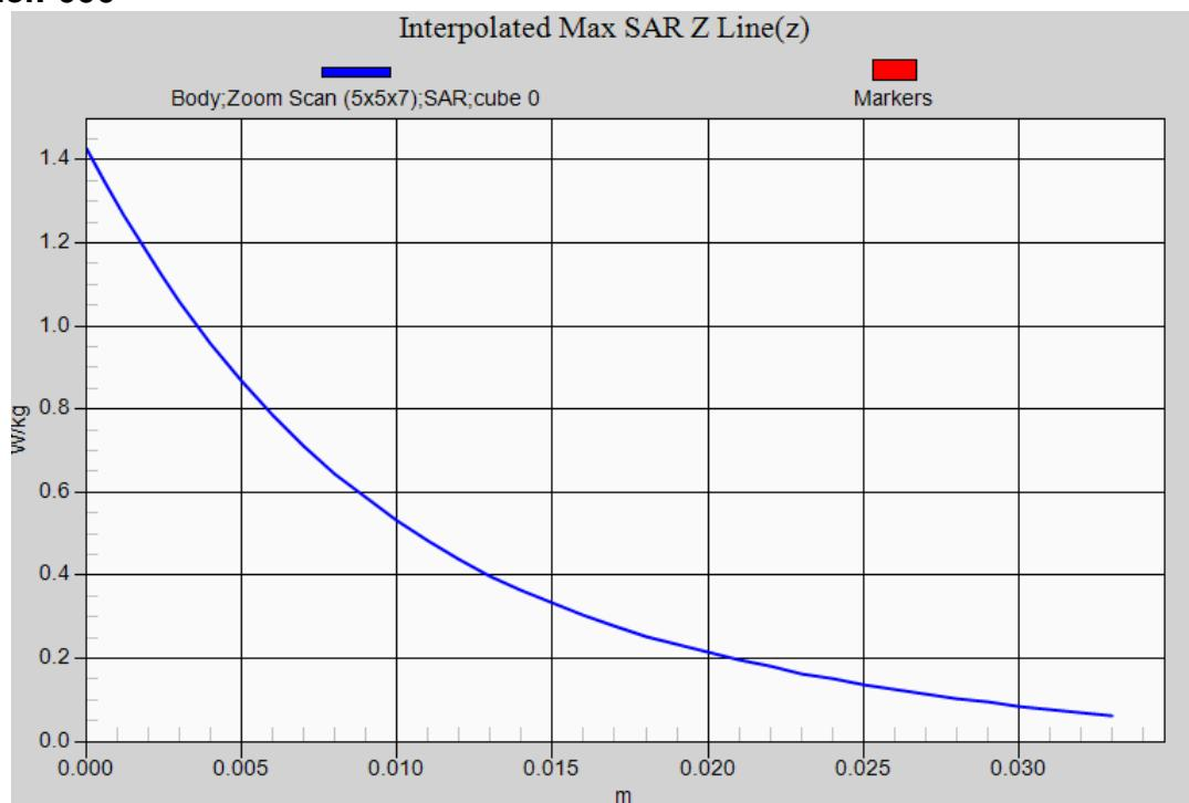
**CDMA BC1 (Limbs SAR) EUT Top (0mm (Pwr OFF)) Z-Axis plot
