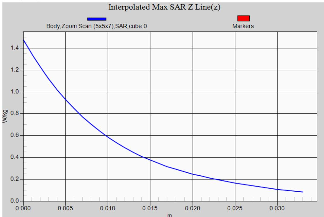
**LTE Band 4 QPSK 1RB (Limbs SAR) EUT Top (0mm Pwr OFF) Z-Axis plot**
