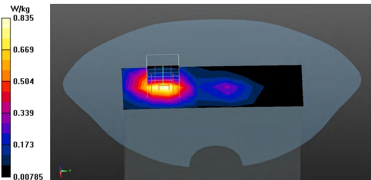
**LTE Band 2 QPSK 1RB (Body SAR) EUT Back (6mm Pwr OFF) Z-Axis plot
