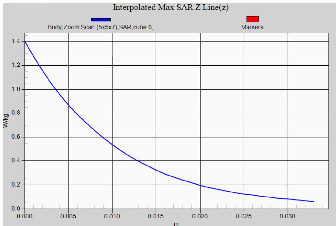
**LTE Band 25 QPSK 1RB (Limbs SAR) EUT Top (0mm Pwr OFF) Z-Axis plot
