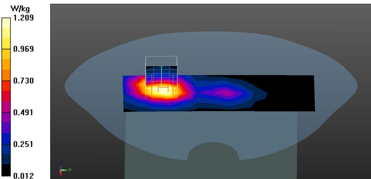
**WCDMA RMC Band 2 (Body SAR) EUT Back (6mm (Pwr OFF)) Z-Axis plot
