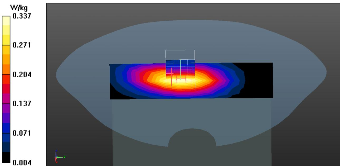
**LTE Band 5 QPSK 1RB (Body SAR) EUT Back (0mm Pwr OFF) Z-Axis plot
