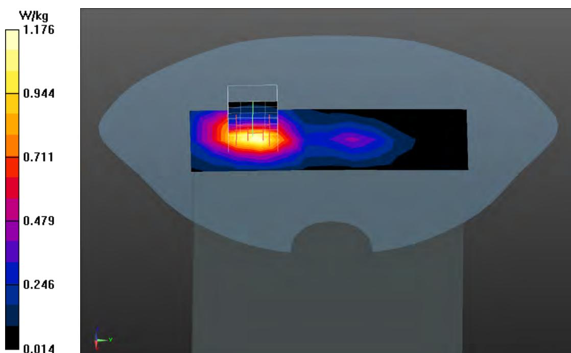
**CDMA BC1 (Body SAR) EUT Back (6mm (Pwr OFF)) Z-Axis plot
