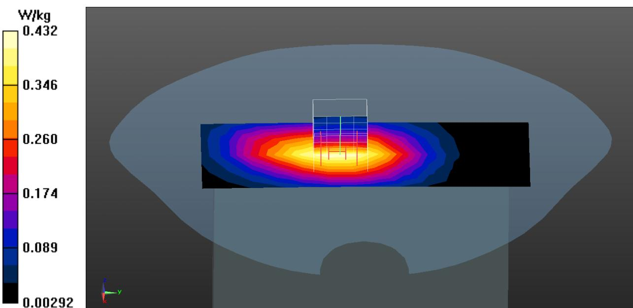
**WCDMA RMC Band 5 (Body SAR) EUT Back (0mm (Pwr OFF)) Z-Axis plot**
