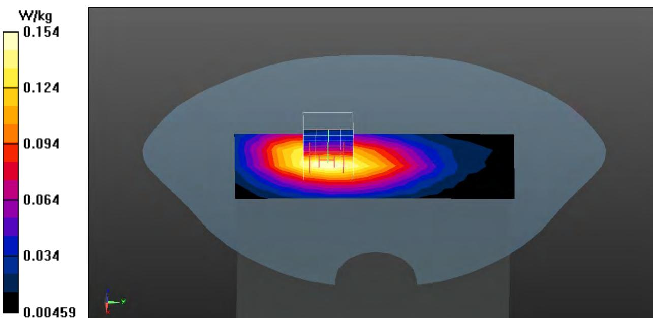
**LTE Band 17 QPSK 1RB (Body SAR) EUT Back (0mm Pwr OFF) Z-Axis plot
