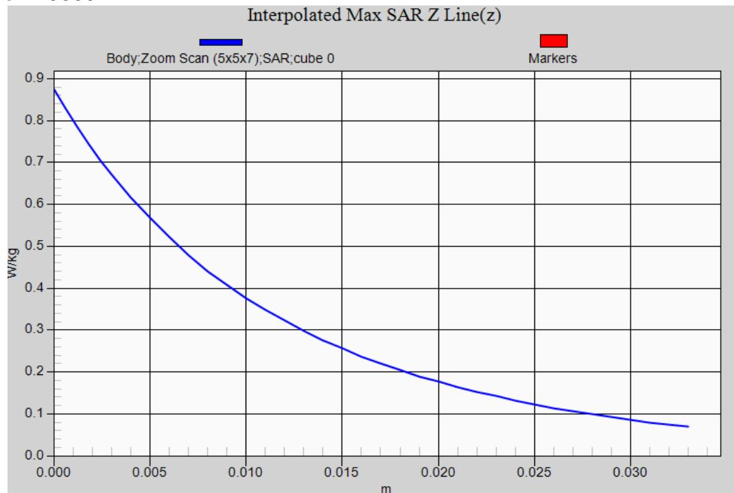
**LTE Band 17 QPSK 1RB (Limbs SAR) EUT Top (0mm Pwr OFF) Z-Axis plot
