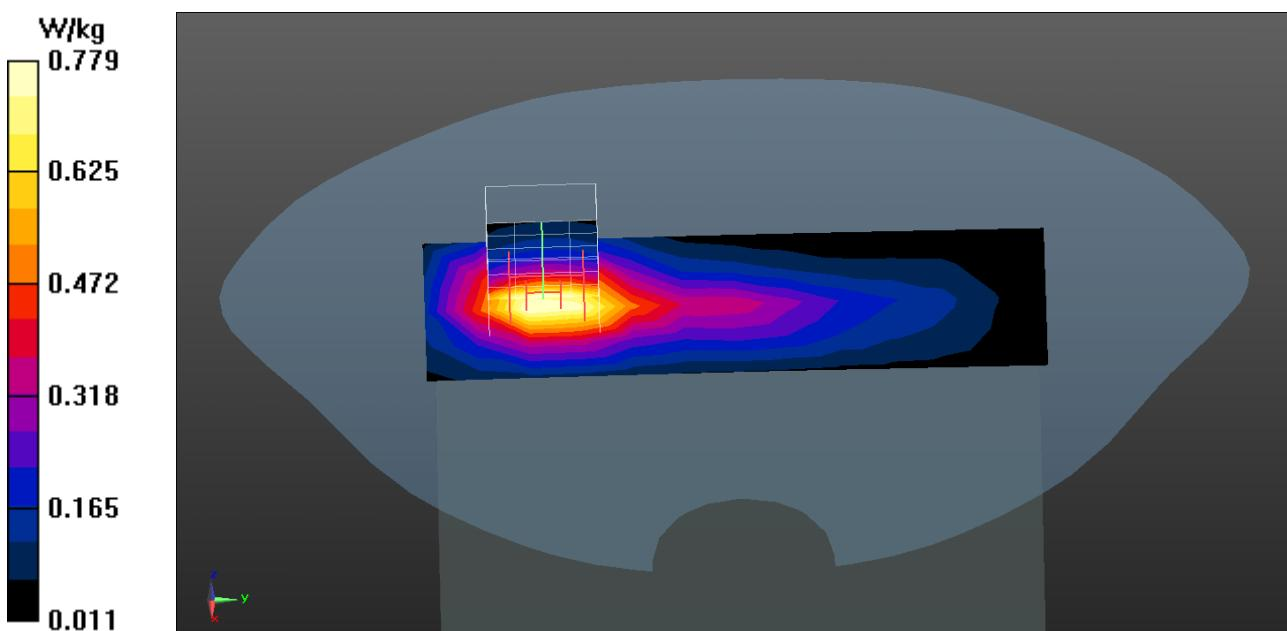
**LTE Band 4 QPSK 1RB (Body SAR) EUT Back (6mm Pwr ON) Z-Axis plot**
