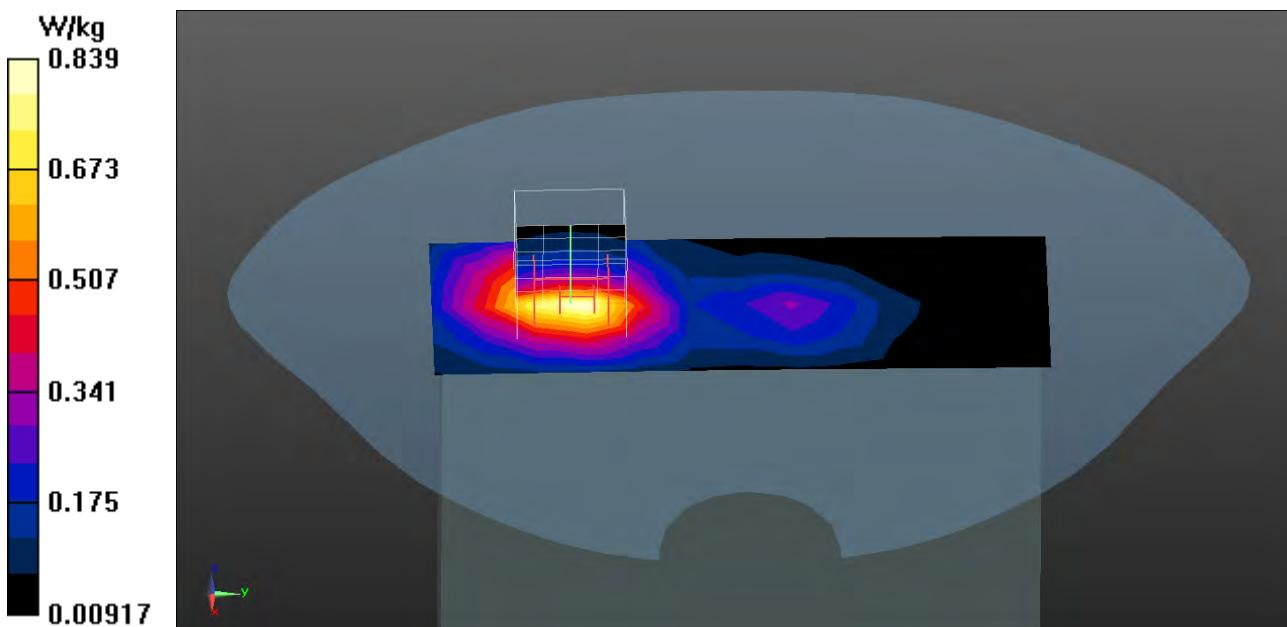
**LTE Band 25 QPSK 1RB (Body SAR) EUT Back (6mm Pwr OFF) Z-Axis plot
