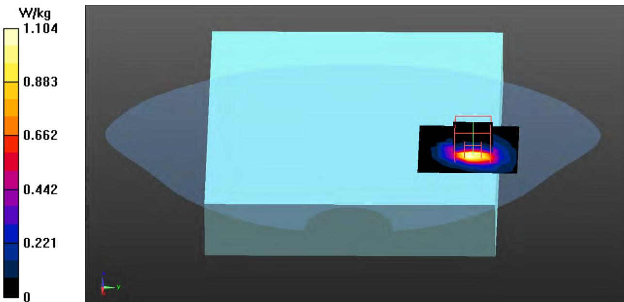
**802.11ac-80M EUT Back (Main Antenna) Z-Axis plot**
