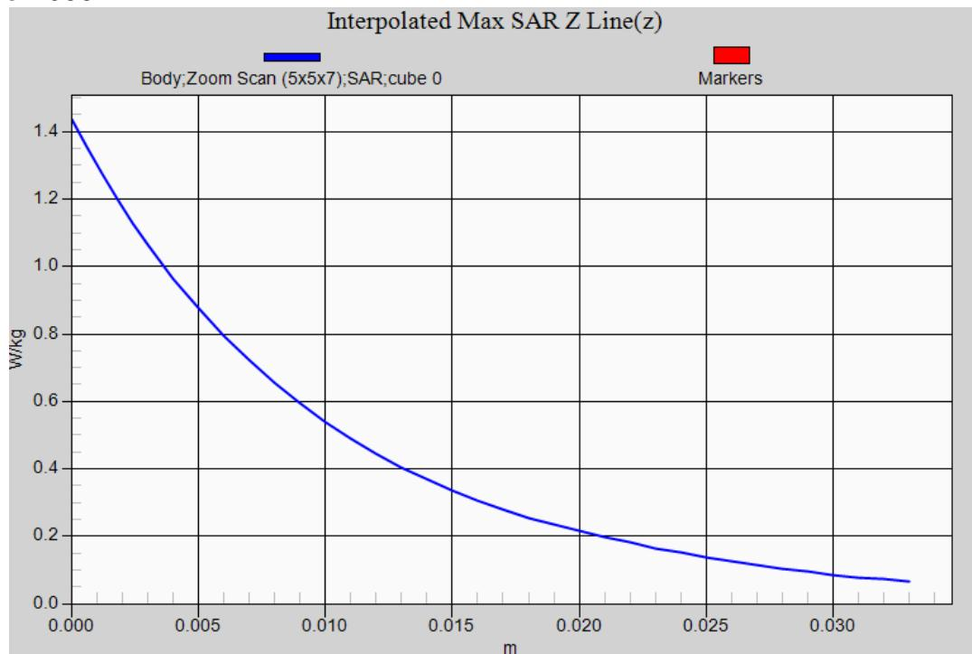
**1xEVDO BC1 (Limbs SAR) EUT Top (0mm (Pwr OFF)) Z-Axis plot
