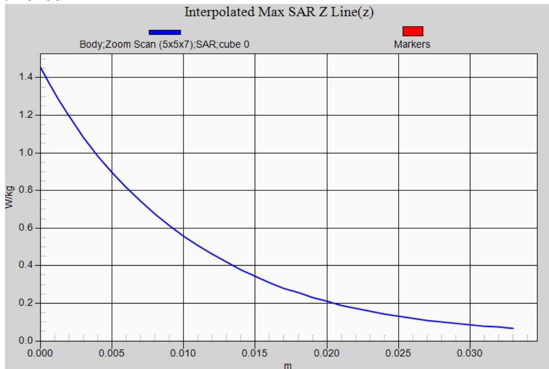
**WCDMA RMC Band 2 (Limbs SAR) EUT Top (0mm (Pwr OFF)) Z-Axis plot
