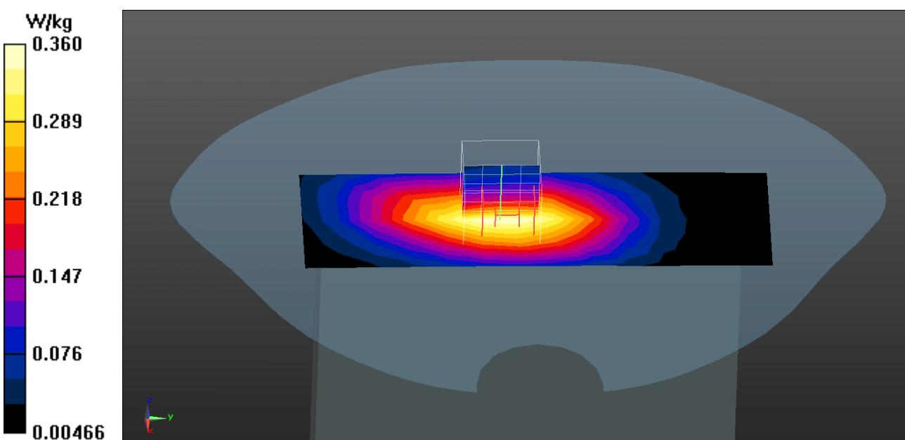
**CDMA BC10 (Body SAR) EUT Back (0mm (Pwr OFF)) Z-Axis plot
