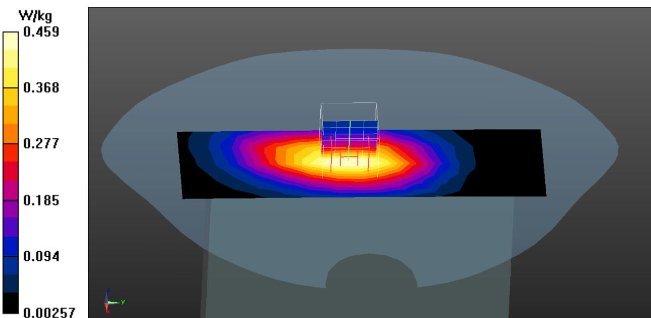
**1xEVDO BC0 (Body SAR) EUT Back (0mm (Pwr OFF)) Z-Axis plot
