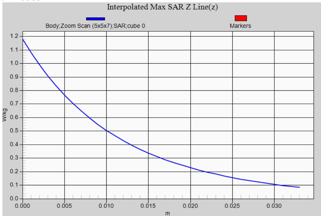
**LTE Band 26 QPSK 1RB (Limbs SAR) EUT Right-side (0mm Pwr OFF) Z-Axis plot**
