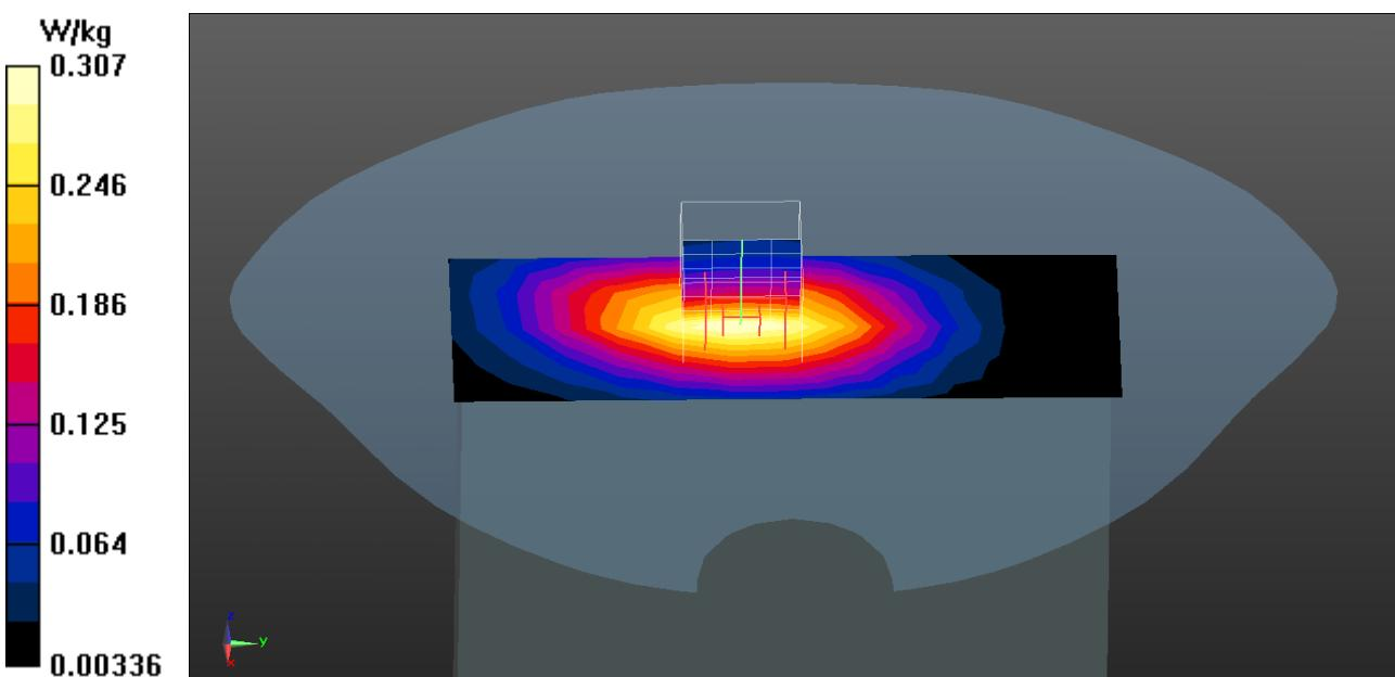
**LTE Band 26 QPSK 1RB (Body SAR) EUT Back (0mm Pwr OFF) Z-Axis plot**
