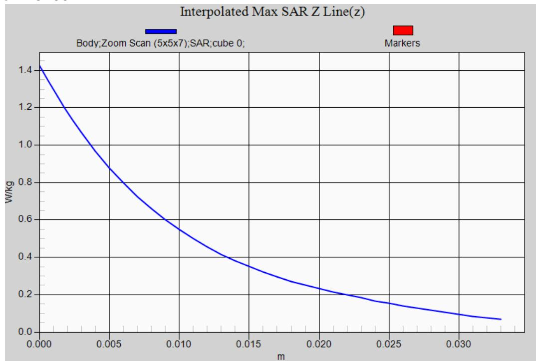
**LTE Band 2 QPSK 1RB (Limbs SAR) EUT Top (0mm Pwr OFF) Z-Axis plot
