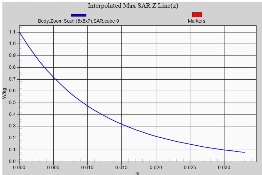
**LTE Band 5 QPSK 1RB (Limbs SAR) EUT Right-side (0mm Pwr OFF) Z-Axis plot
