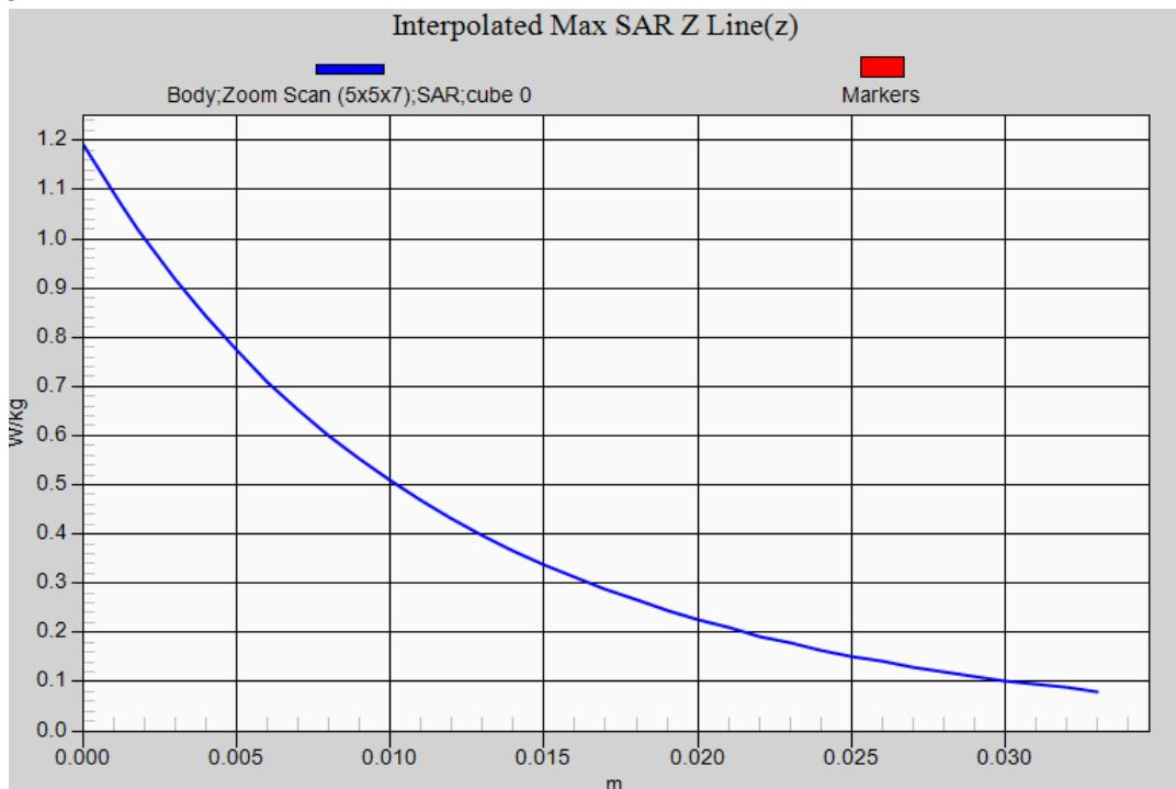
**1xEVDO BC0 (Limbs SAR) EUT Right-side (0mm (Pwr OFF)) Z-Axis plot
