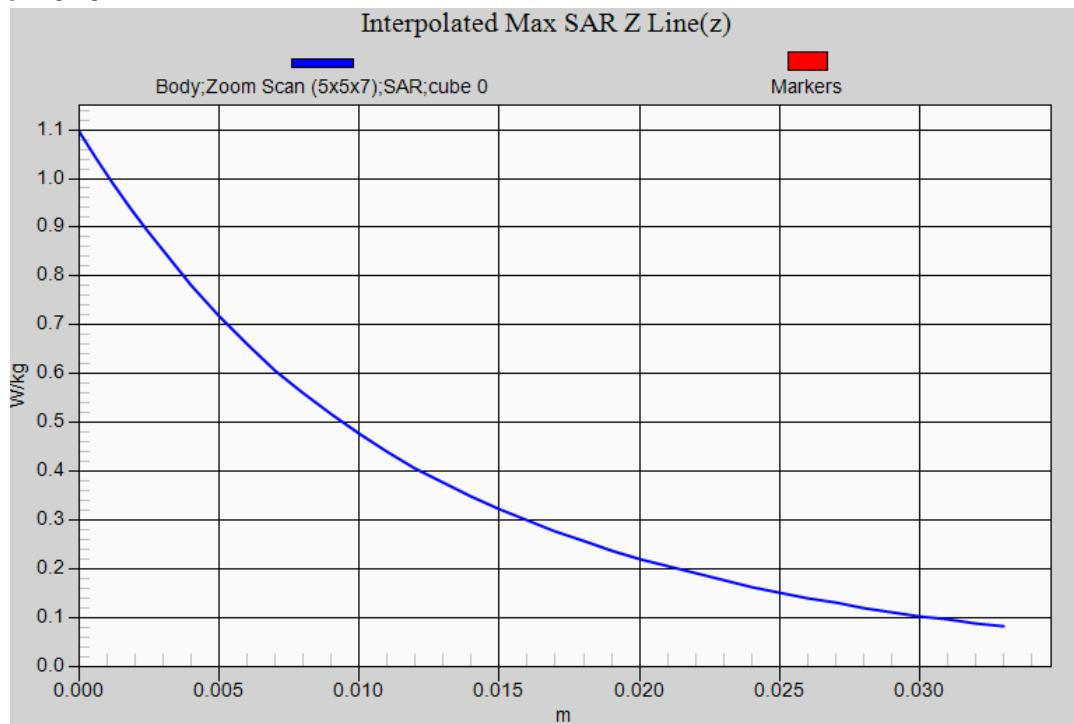
**CDMA BC10 (Limbs SAR) EUT Top (0mm (Pwr OFF)) Z-Axis plot
