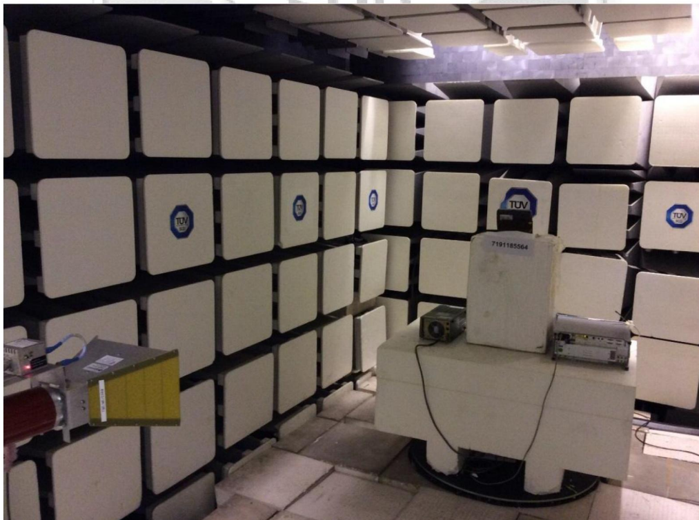
Out of Band Emissions Test Setup (Rear View)
