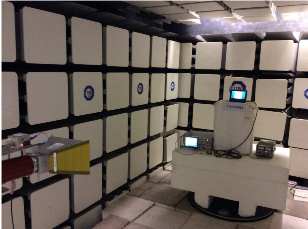
Out of Band Emissions Test Setup (Front View)
