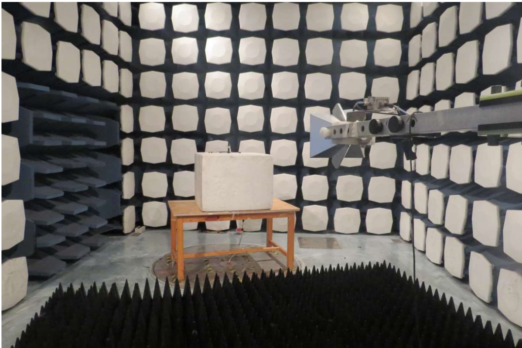
Picture 1: Radiated Spurious Emissions Test setup
