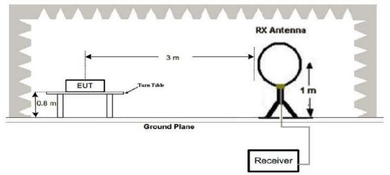
(2) Radiated Emission Test-Up Frequency 30MHz~1GHz
