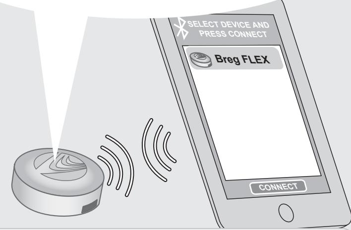
On the mobile device, go to tools and ensure that the Bluetooth function is turned on and the sensor is available for pairing (syncing).
