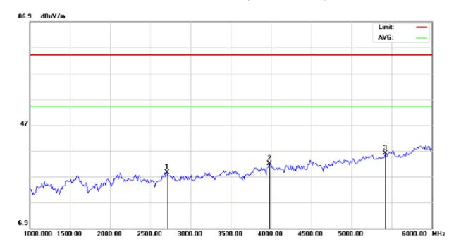
Site: site #1 Limit: FCC Class B 3M Radiation above 1GHZ(PK) Polarization: Vertical
