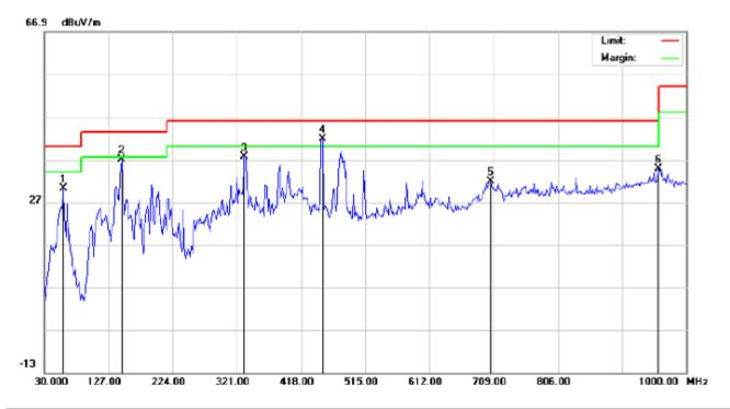
Site: site #1 Polarization: Horizontal Temperature: 22.8 Limit: FCC Class B 3M Radiation Power: AC 120V/60Hz Humidity: 53.8 %
