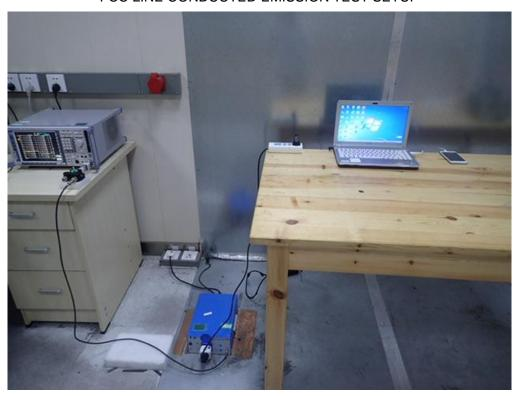
FCC RADIATED EMISSION TEST SETUP
