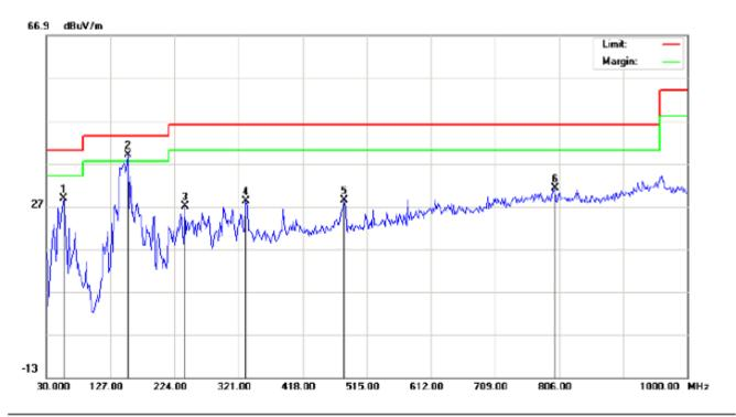
Site: site #1 Polarization: Vertical Temperature: 22.8 Limit: FCC Class B 3M Radiation Power: AC 120V/60Hz Humidity: 53.8 %
