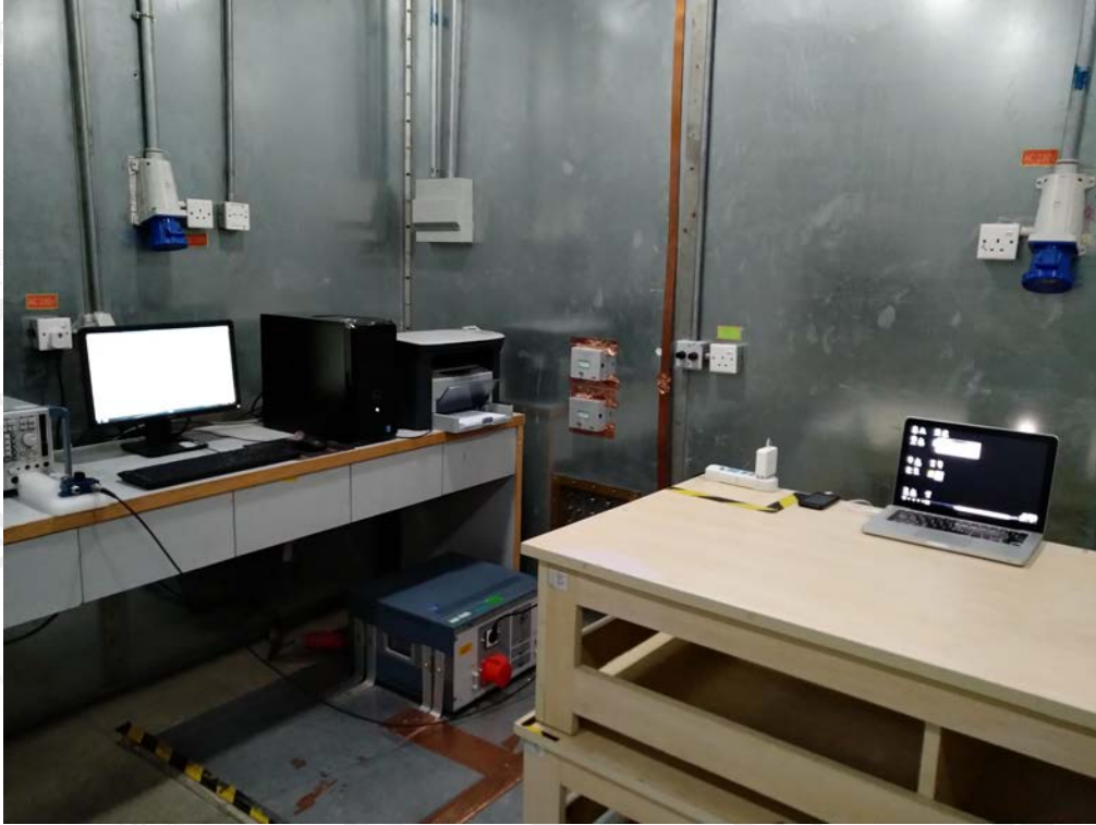
FCC RADIATED EMISSION TEST SETUP
