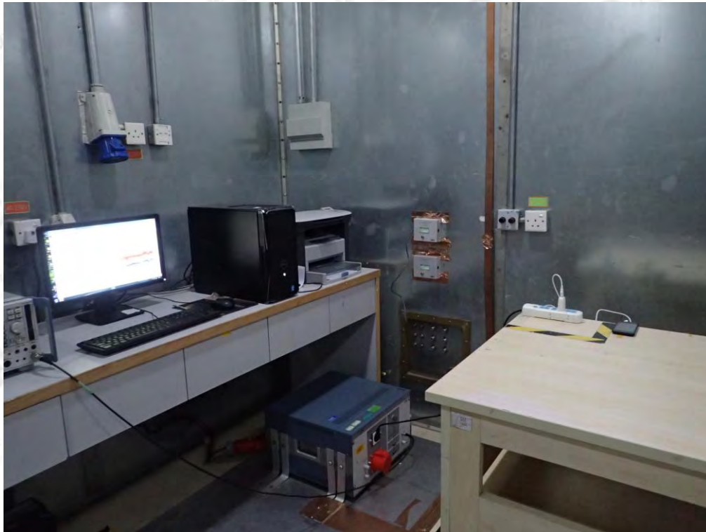
RADIATED EMISSION TEST SETUP
