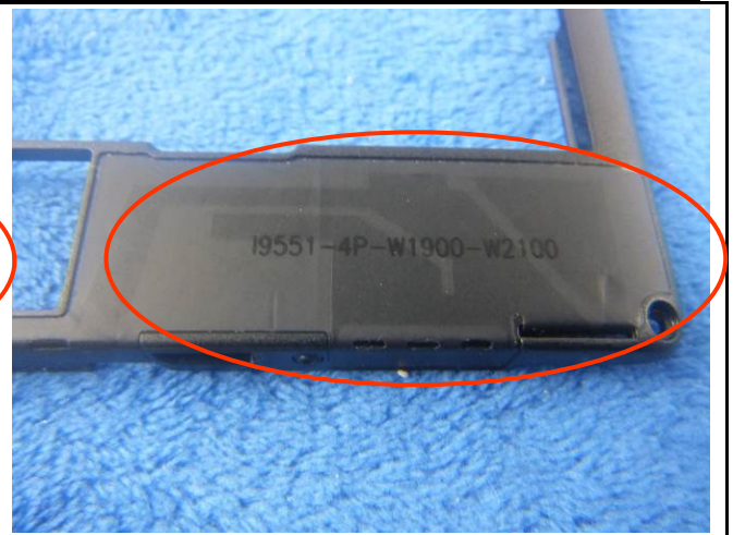
GSM/PCS/UMTS-FDD Antenna View
