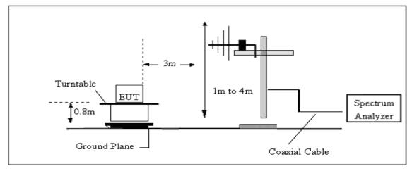
(A) Radiated Emission Test-Up Frequency 30MHz~1GHz
