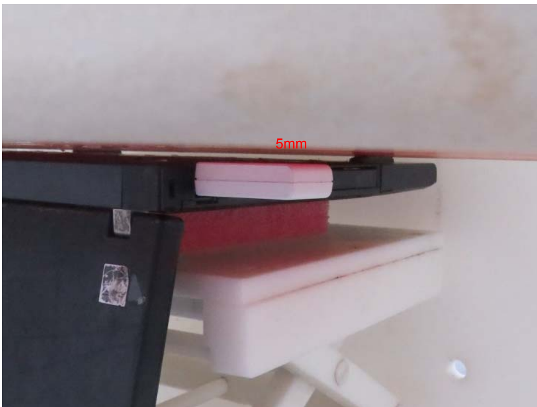
Picture 6: Front Side, the distance from EUT to the bottom of the Phantom is 5mm
