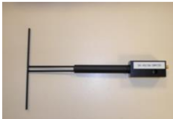
Figure 1 – MVG COMOSAR Validation Dipole
