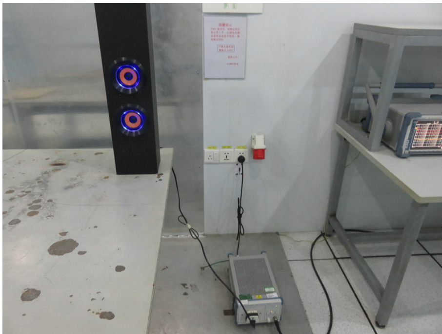
1 Photo of Power Line Conducted Emission Measurement
